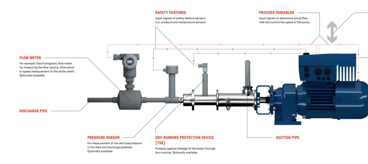
The SDP features an integrated PLC to enable stand alone operation in, for example, distributed control systems (DCS). Set points are entered and sensors on the pump feed back operating conditions to the integrated PLC. Complex implementation into higherlevel controllers is no longer required. This simplifies automation system integration and reduces the cost of installation and maintenance.
